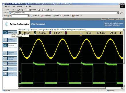
Figure 3. Remotely display and control the oscilloscope from any java-enabled web browser over the LAN interface
